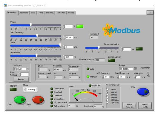
7. After pressing the button RESCAN you have all parameters and settings from the generator uploaded in Labview software.
