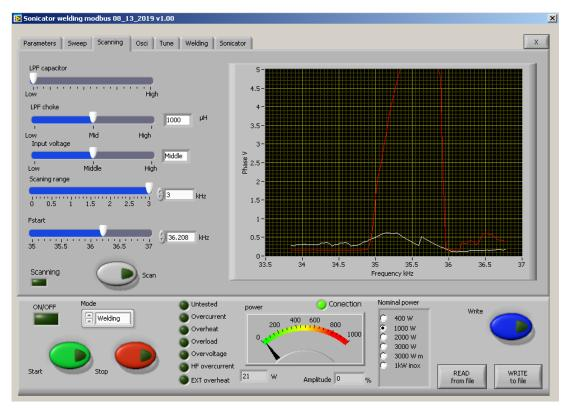
The generator has Scanning function which is very powerful instrument for the operator. Here you can discover the phase and current characteristic of the exact load. It is shown graphically in an window in Scanning tab.
