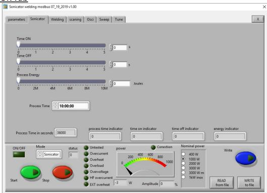
**Time ON** – Set the operation time of the generator in Sonicator mode.
